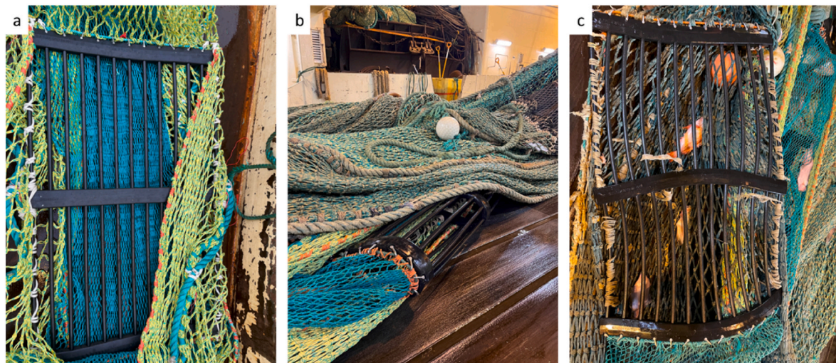
Fig. 4. Pictures of a grid in the new flexigrid section (a), a grid in the used flexigrid section deformed on deck (b), and a grid in the used flexigrid section laying on deck (c).
