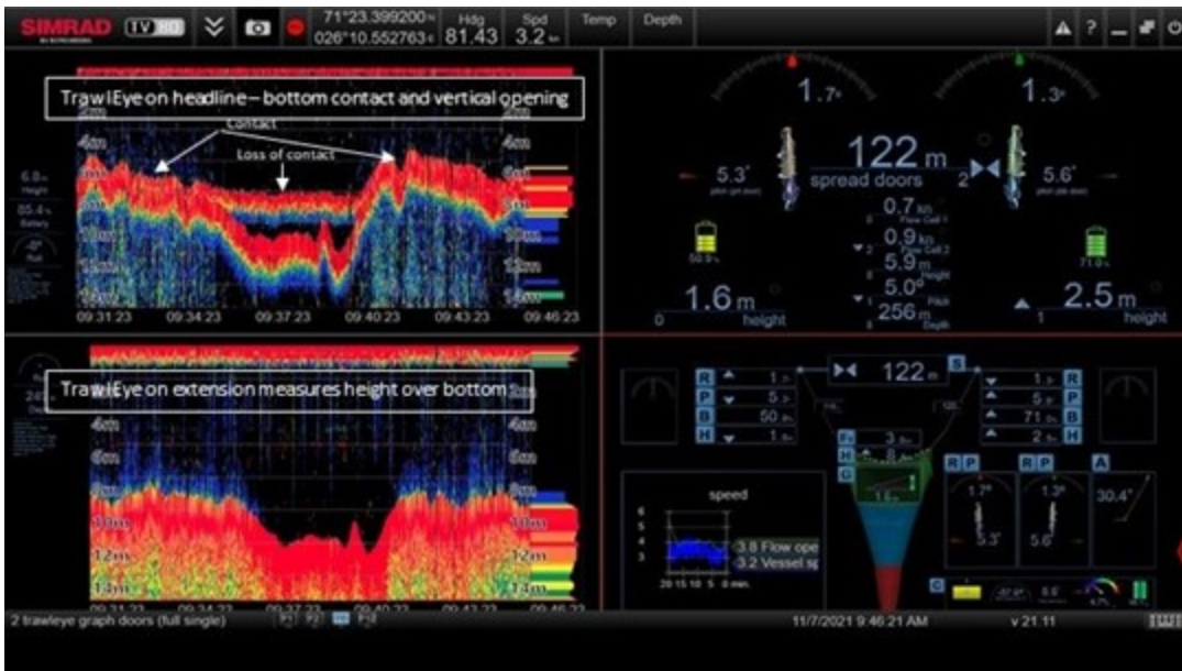
Figure 6 . Screen shot from TV80 (KM) software. Showing the TrawlEye echograms (bottom contact and height over seabed and data from door and flow sensors on the right).
