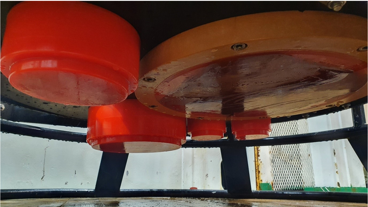
Figure 16 .2. Acoustics-equipped probe ('TS-probe') as suspended by a reinforced electric-optic wire for live communication and data viewing. TS-probe contains four broadband transceivers (black cylinder in the middle) that are coupled to the transducers mounted on a motorized plate (bottom). Probe was operated at 100-300 m depth (Image credit: Rokas Kubilius/Institute of Marine Research).
