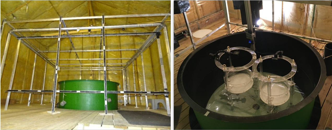
Figure 5. Magnetic orientation testing facility (MagLab). The cube coil (left) allows one to change the direction and intensity of the ambient magnetic field. Two testing arenas were used in the study (right). Each arena was lined with plankton mesh and was fitted with a camera. Four individual fish were tested per trial (two fish per area).
