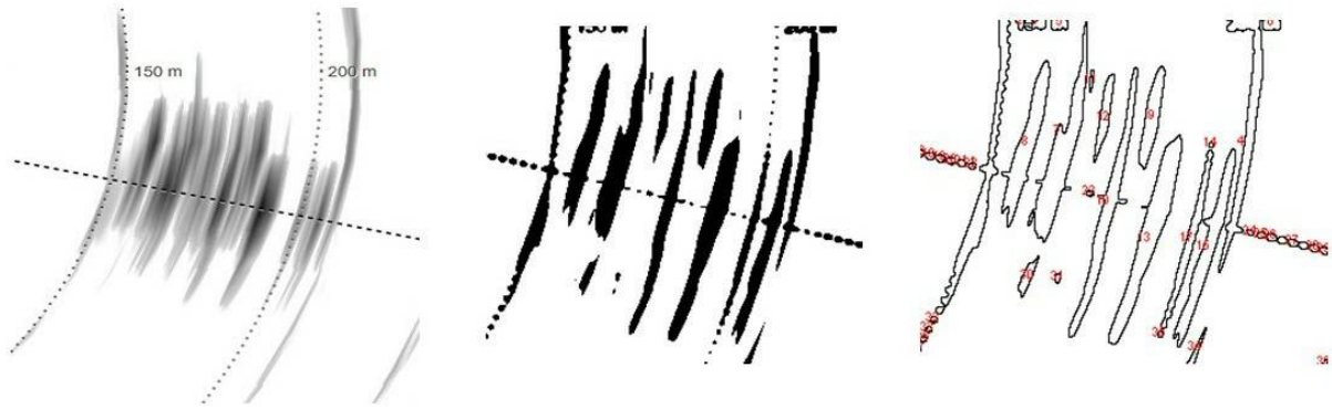
Figure 15. Example of using autothresholding in image J to automatically detect and extract BFT echoes and count the number of individuals. The image is first converted to binary, then a threshold is applied and finally borders of the thresholded parts are detected and the number of shapes counted.
