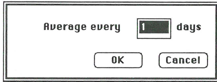
Fig. 38. Giving the number of days to average increment size data over. The default number is 1.
