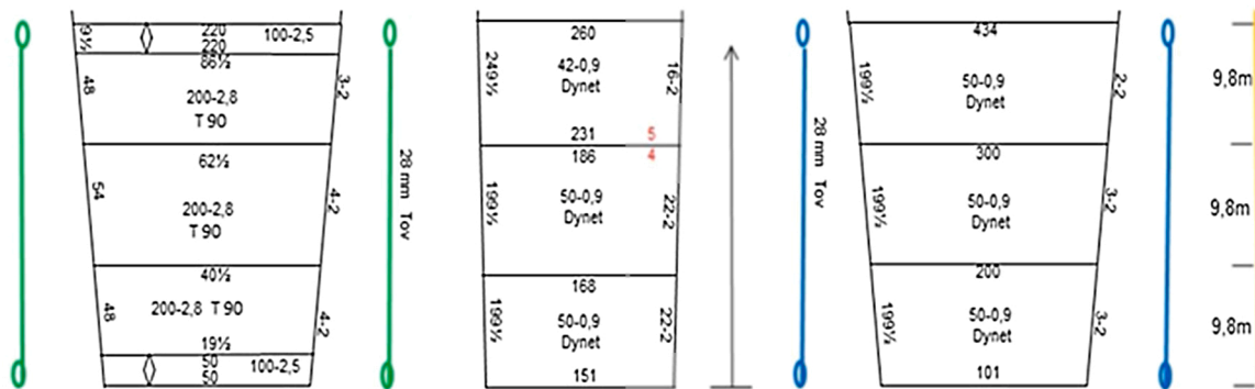
Fig. 3. Technical specifications of the belly sections where the 200 mm T90 mesh panel was inserted. From left to right: top, side, and bottom panels.
