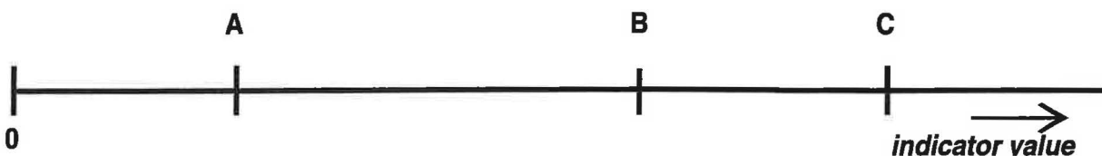
Fig. 3.2 An indicator yardstick. A: actual value, B: target value, C: reference value.
