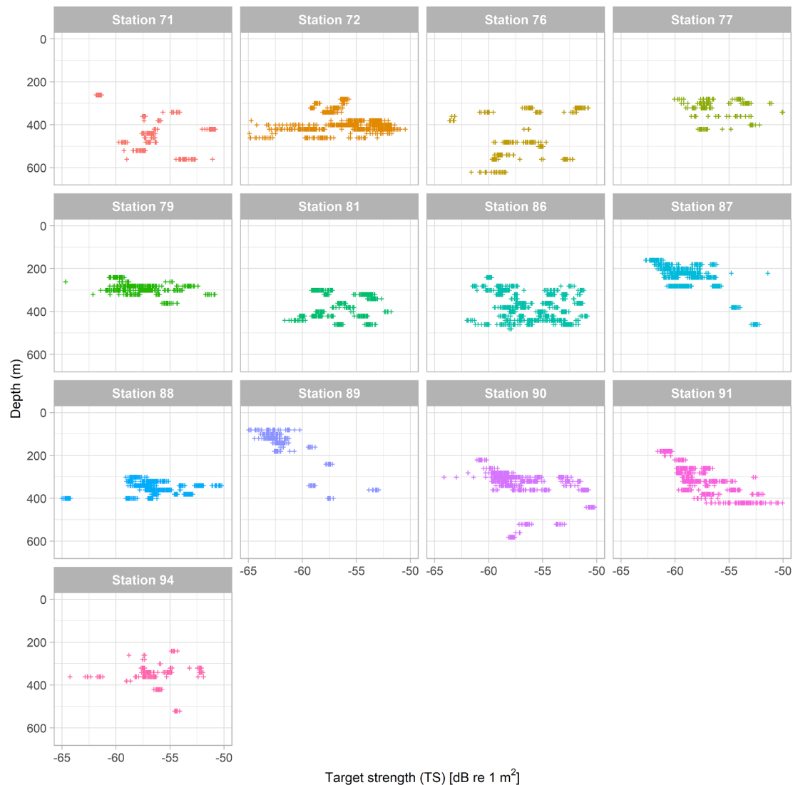
Fig. 4. Target strength (TS) detections for mesopelagic fish by Station. The plots show beam compensated TS (in dB re 1 \text{ m}^2 ) over depth (m) for the stations that registered > 125 detections per station.
