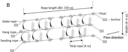
Fig. 4.5 Longline culture in China (above); Schematic diagram of longline culture in China (below)
