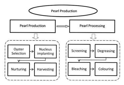
Fig. 5.7 Diagrammatic representation of the stages of pearl production
