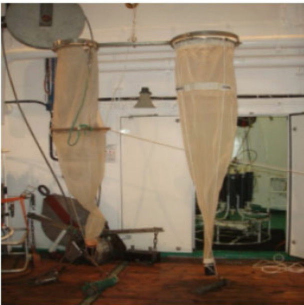
Figure 8. Set up of double-net configuration (in the picture a combination of a Juday and a WP2 net).
