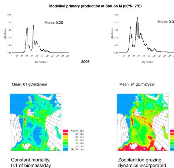
Phytoplankton biomass was simulated by a newly developed model, based on a ROMS physical model and a modified NORWECOM model for phytoplankton, and linked with the zooplankton model.
