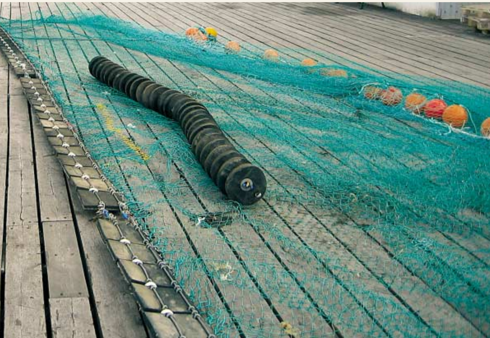
Bottom trawl with sheering ground gear.
