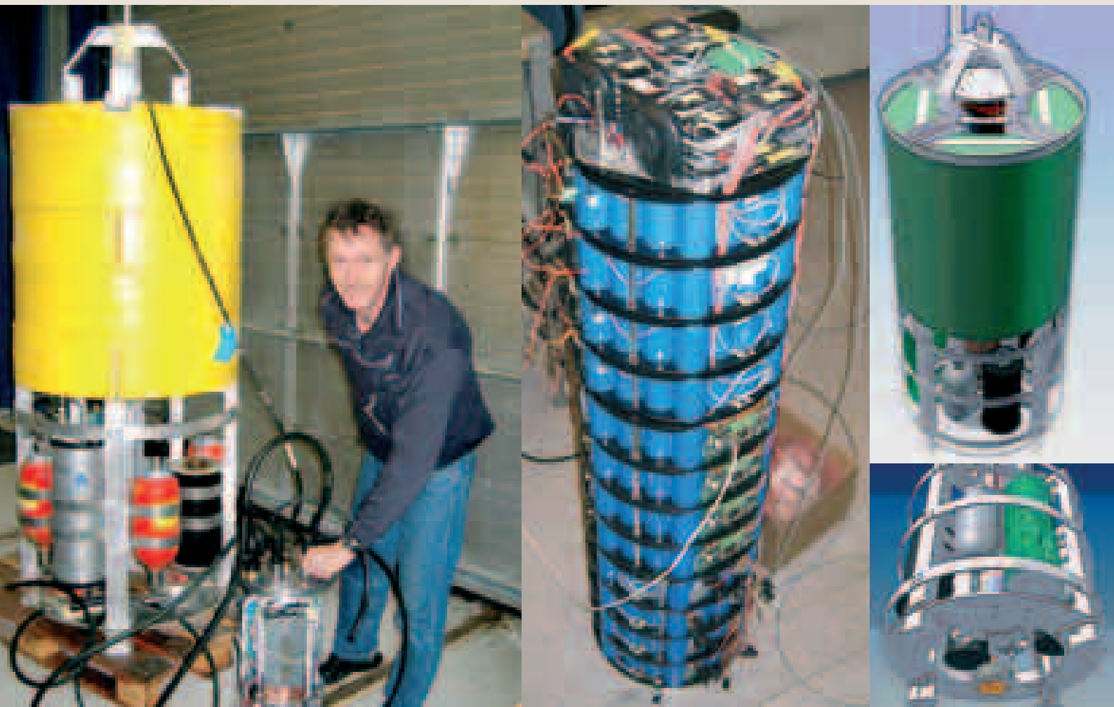
Specially developed battery, artificial buoyancy and antenna to Iridium satellite phone, tolerating pressure to 1000 m depth.
