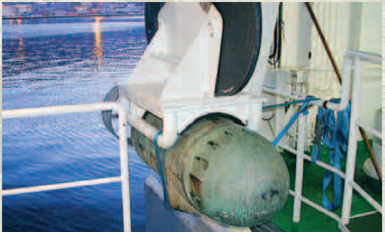
Deployment mechanism for the towed body, on the new “G.O. Sars”.
