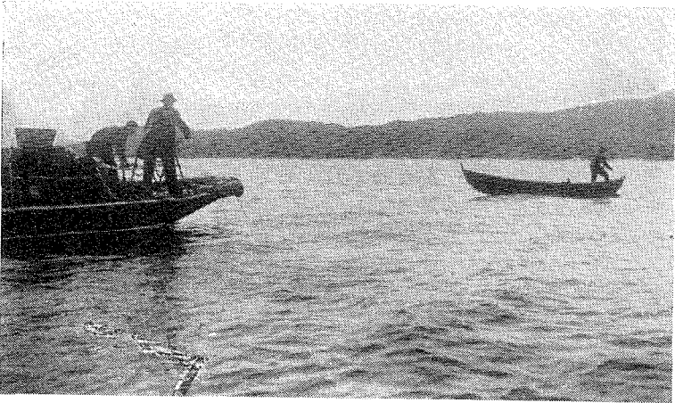
Fig. 32. Skjellplogen varpes inn. En mann er ute i «lettebåten». Fot. A. Wollebæk. The dredge is being warped in. Note the man in the smaller boat. He elevates the dredge with a rope when it sticks to the bottom.
