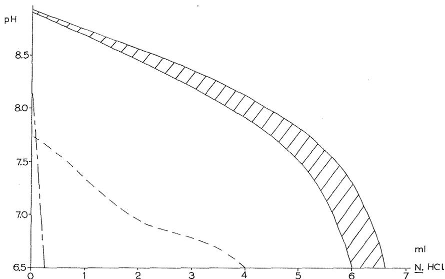
Fig. 1. pH versus ml N hydrochloric acid added to 1 g of buffer dissolved in 100 ml of seawater. ——— Buffer curve of seawater. - - - - Buffer curves of borax, "tris", glycyglycine and taurine lie within this envelope.
