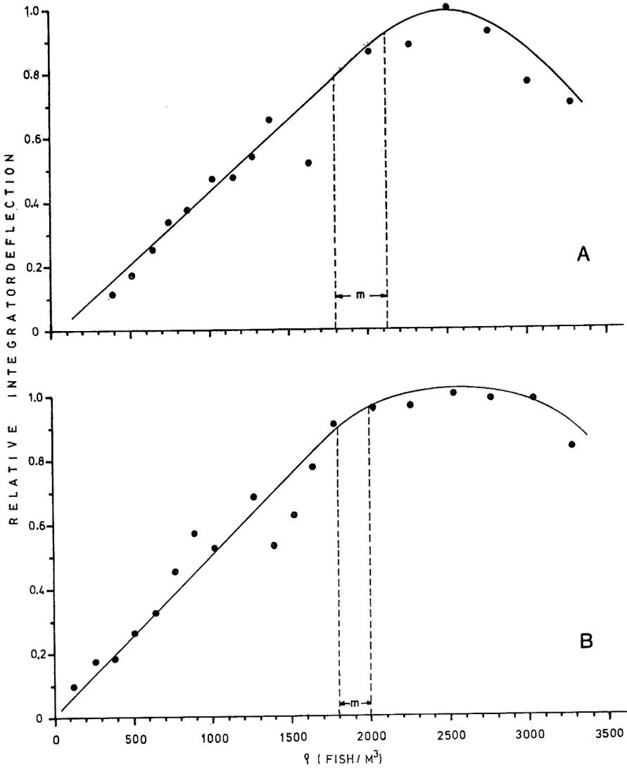
Fig. 7. Observations of relative integrator deflection on densities of sprat at 38 kHz.
