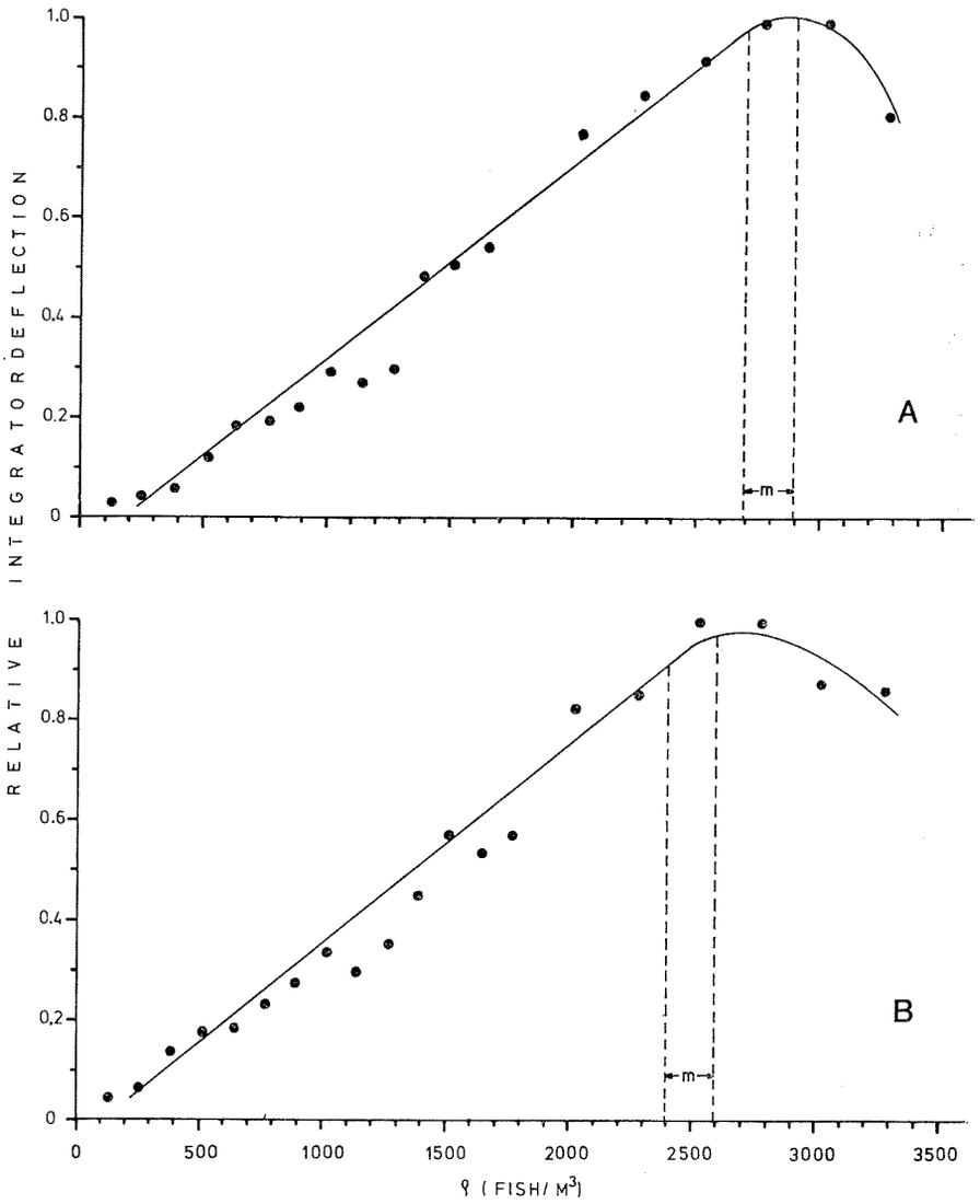
Fig. 8. Observations of relative integrator deflection on densities of sprat at 120 kHz.
