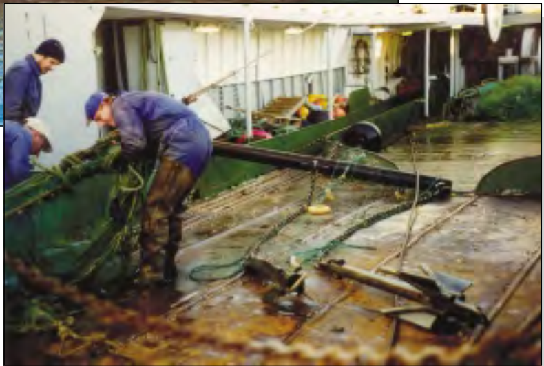
Figur: 5.3.3 Sokneapparat for garnrydding. The device applied for retrieving gillnets.
