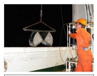
Sampling of bottom sediments using van Veen grab.
