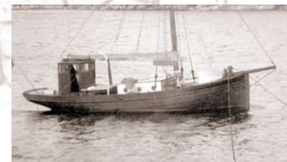
Length: 40 ft Built: 1914, in Germany In 1929 new 24 Hp Rap-motor
