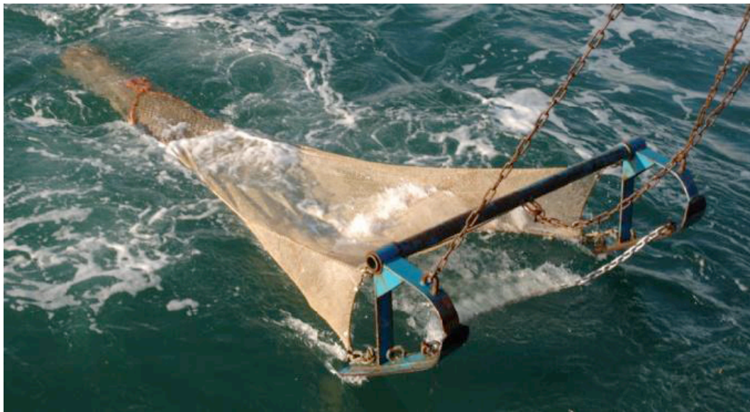
Fig. S5. Dredge (Plot Sampling). Dredges are used to catch endo- and epibenthos. Depending on the surface, dredges can dig into the sediment or scrape organisms off hard surfaces. Photo: Senckenberg, Sven Traenkner.
