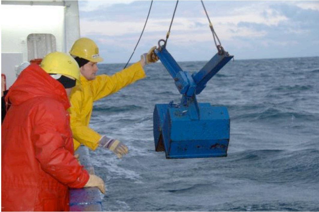
Fig. S2. The Van Veen grab (Plot Sampling) is used for endobenthos, it is more suitable under rough weather conditions than box corers. Photo: Senckenberg, Sven Traenkner.
