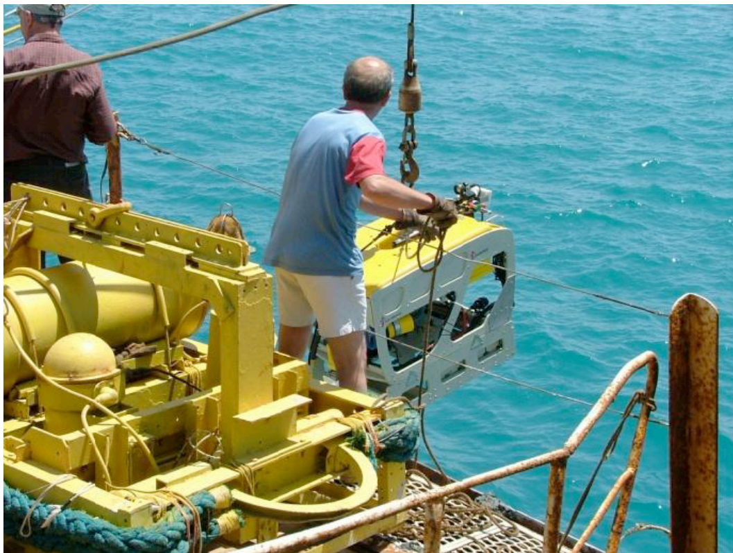
Fig. S7. Remotely Operated Vehicle (ROV) "Cherokee" (Plot Sampling). This underwater vehicle dives 1000 m deep, is equipped with cameras and can collect samples. Photo: MARUM, Universität Bremen.
