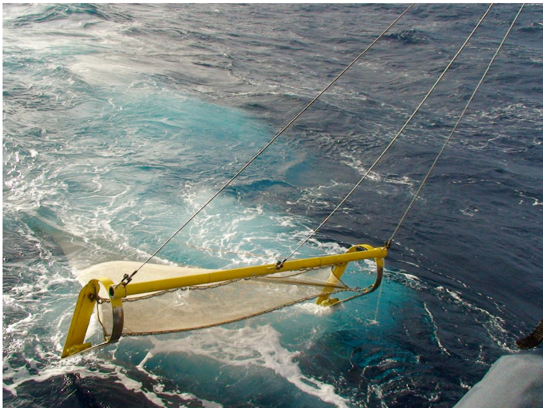
Fig. S3. Agassiz trawl (Plot Sampling). This demersal trawl is used to catch epibenthos. In advantage to other trawls the Agassiz trawl works on either side when landing on the seafloor, which improves catchability. Photo: Hartmut Arndt.
