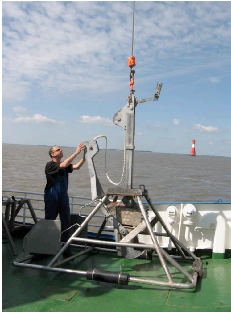
Fig. S1. The box corer (Plot sampling) is used for endobenthos, the major advantage is to collect sediment blocks with negligible disturbance. Recovered onboard, the box can be detached from the frame for subsampling and further analysis. Photo: Senckenberg, Sandra Vöge.
