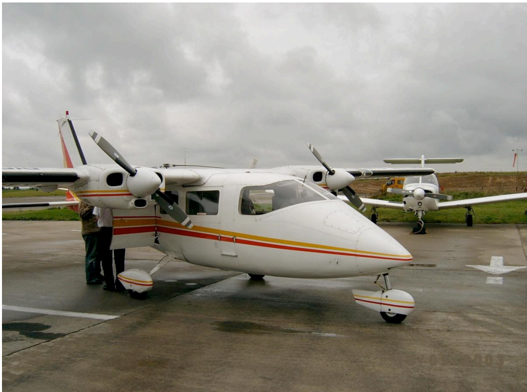
Fig. S9. Typical high-wing twin propeller aircraft used in aerial surveys for strip transects (Plot Sampling) or line transects (Distance Sampling) of marine mammals, seabirds, large fish, jellyfish etc. Photo: Tom Doyle
