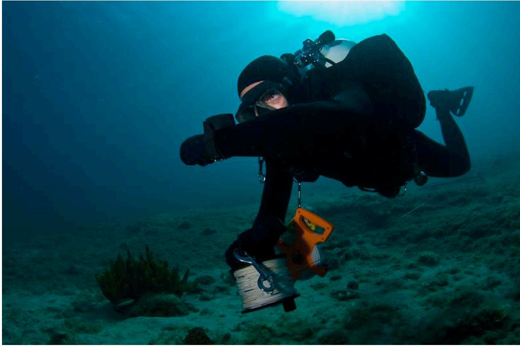
Fig. S14. In strip transects (Plot Sampling) or line transects (Distance Sampling) in underwater visual surveys, the simplest and best way to define a transect is by delineating the center-line. Here the diver-researcher deploys a nylon line with a use of a diving reel; an underwater compass is used to position a straight line in the desired direction of the transect. Photo: Yiannis Issaris.
