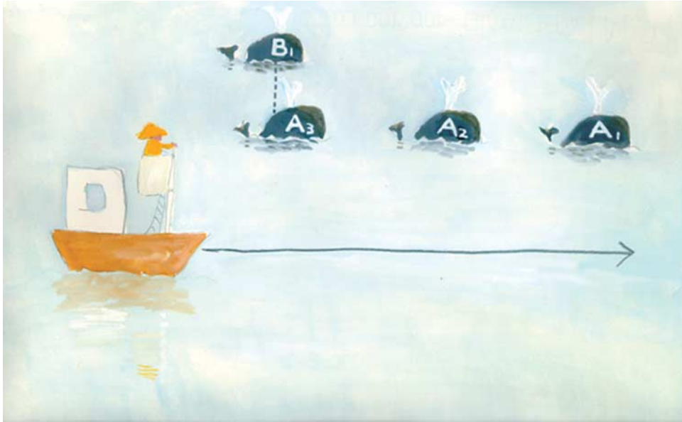
Fig. 2. Double-platform shipborne sighting surveys. Observer platform A is placed in the barrel as shown, and observer platform B (not shown) is placed at the wheelhouse roof. The depicted scenario involves a single whale making three surfacings, which are all detected by platform A. Platform B sees only the last surfacing. Thus, A1 is the initial sighting of the whale, whereas A3 and B1 form a duplicate sighting, as indicated by the broken line. Because of measurement error in distance and sighting angle, the recorded relative positions of A3 and B1 differ. In the statistical analysis, the second and third surfacings form Bernoulli trials for platform B. (Artist: Åsa Gan Schweder.)
