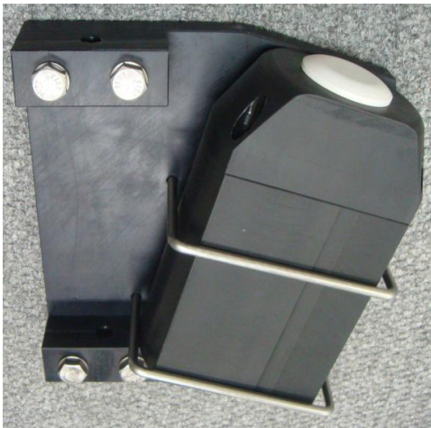
Figure 4. The EchoTag, example of a 190-kHz single-beam echosounder and temperature logger that can be mounted on moorings, and capable of delivering profiled volume backscattering strength from its location at 150 m to the sea surface for durations of greater than one year.
