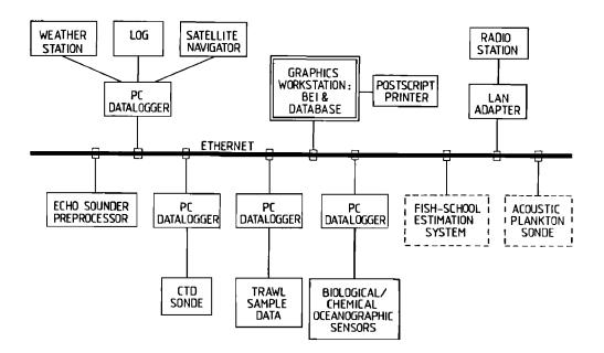
FIG. 1. Data network for research vessels.
