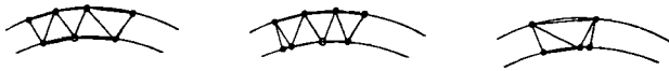
FIG. 2. Illustration of triangulation by angular affinity. Solid circles represent points obtained by the standard homeomorphic mapping. Open circles represent interpolated points.
