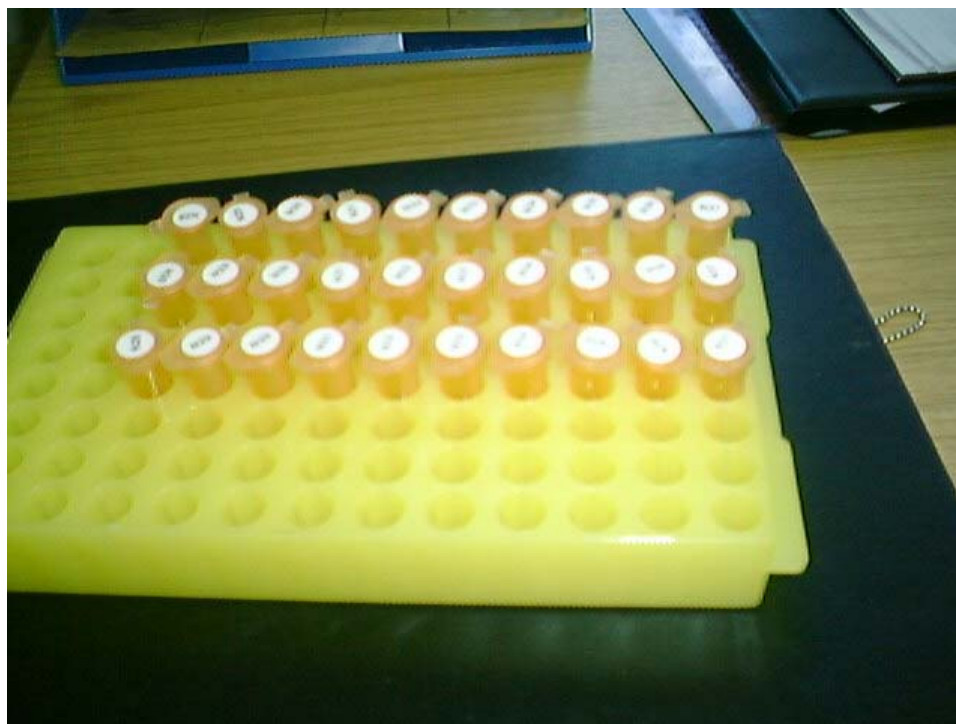
Figure 3.4.6.2 Picture of a rack holding Eppendorf like tubes for 10 fish with 3 replicates identified by spot labels on the lids. During storage a lid fits on top of the rack to keep the tubes in order during transport
