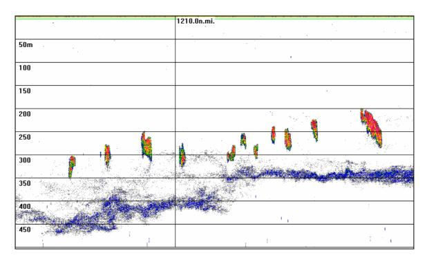
**Figure 3.3.3** Echogram showing schools of Norwegian spring spawning herring observed by R/V *Magnus Heinason* in the northern part of the Faroese EEZ in late May 2003.
