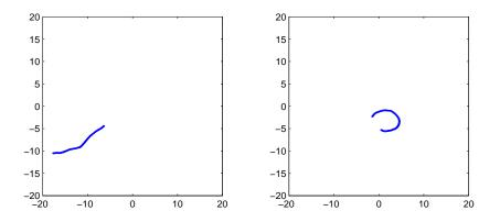
Figure 2: Trajectories of a particle simulated with the model (7). Left panel:  $A = A_1$ . Right panel:  $A = A_2$ . With  $A_2$  the trajectories have a tendency to turn counter-clockwise; with  $A_1$  turns are rarer and have no preferred direction.
