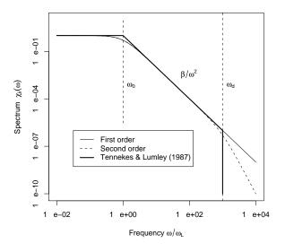
Figure 1: Lagrangian time spectrum of velocity in stationary homogeneous isotropic turbulence. The form in the inertial subrange, between  $\omega_0$  and  $\omega_d$ , is universal and derived from similarity theory. Below  $\omega_0$  the form is flow dependent; to make progress in general theory one chooses the simplest possible form. Above  $\omega_d$  viscosity becomes important and the roll-off becomes steeper; if one wishes to include the effect it may be done with a secondorder model.
