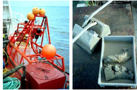
Ground-truthing: (left) A benthic sledge fitted with u/w video and stills. The position of the sledge relative to the ship is recorded in "real time" using acoustic tracking equipment (ORE LXT System). (right) A Van-Veen grab is used to collect samples for Particle Size Analysis.
