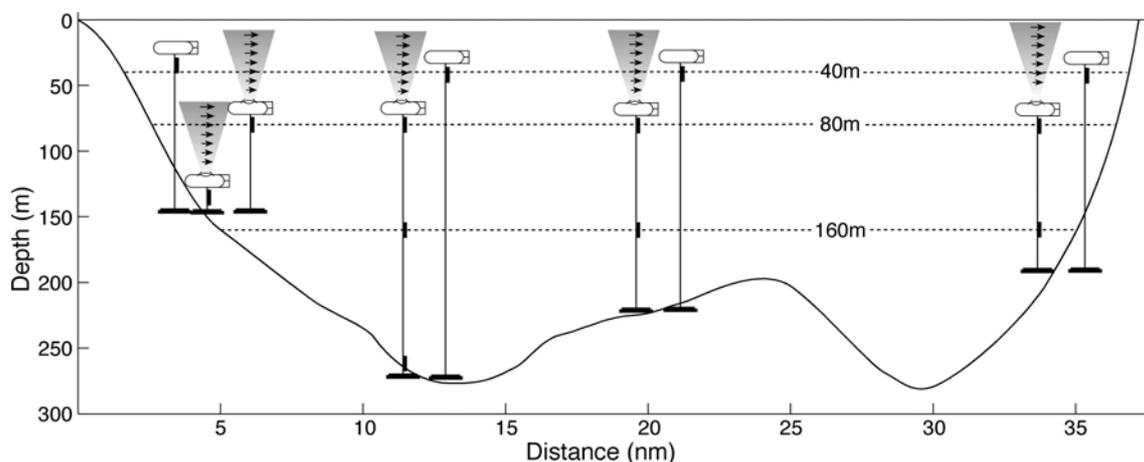
**Figure A.D.1.** Mooring array of August 2001 to August 2002 in Lancaster Sound.
