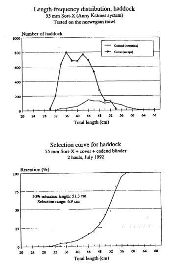
Figure 9. Haddock (<u>Melanogrammus aeglefinus</u>). Length-frequency distribution and selection curve obtained with the Sort-X system used on board "Poljamoje Sijanije" during the joint experiments. The haddock experiment was made with a norwegian trawl on board "Anny Krämer" in the period 26-29 July 1992 along the Norwegian coast.
