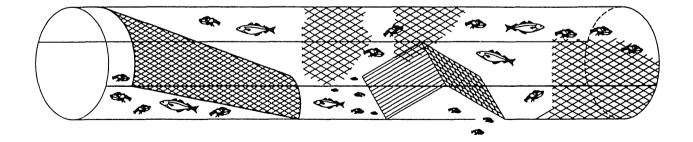
Figure 8. Grid system for releasing small nephrops
