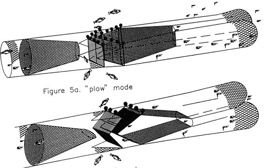
Figure 5b. vertical mode Figure 5. V-grid system for releasing small shrimp and fish of all sizes
