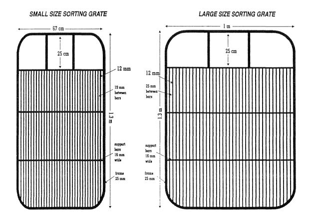
Figure 2: A Diagram of the Large and Small Shrimp Size Sorting Grates.
