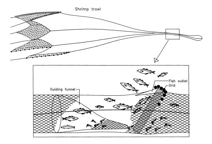
Figure 1. Nordmøre grid shrimp-fish separating system
