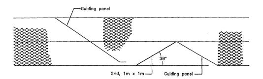
Figure 4. Bottom-mounted grid & extension
