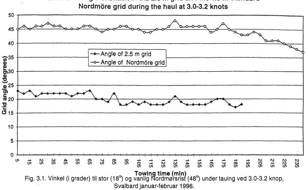
Measured angle of attack of the 2.5 m grid and the 1.5 m standard
