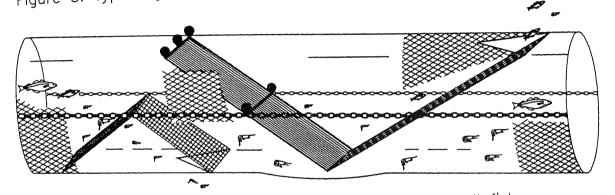
Figure 4. Grid system for releasing small shrimp & small fish
