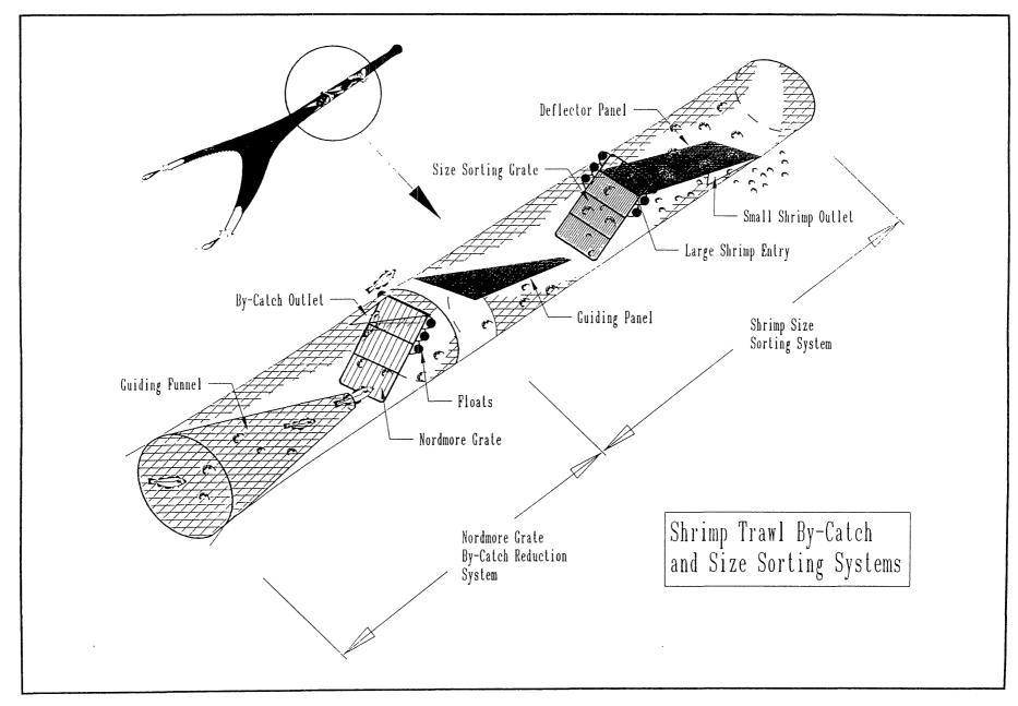
Figure 3: A Diagrammatic Representation of the Size Sorting Grate and its Mechanics.
