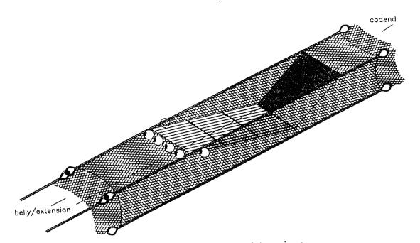
Figure 3. Typical grid installation for Danish seines
