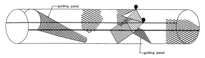
Figure 6. Grid system for releasing small shrimp and all fish
