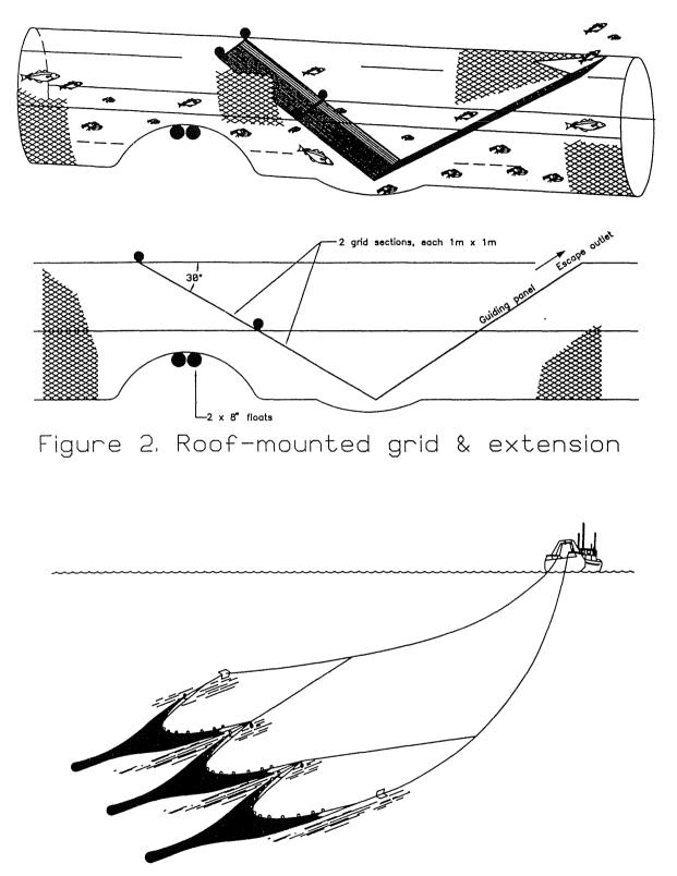
Figure 3. Schematic of triple trawl system
