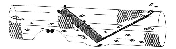
Figure 7. Grid system for releasing small nephrops and small fish
