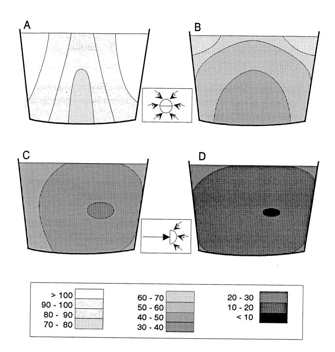
Fig. 1. Isolines of light intensities (relative values) measured in tanks with white walls and white bottom. A: clear water, 360°; B: green water, 360°; C: clear water, 180° (horisontal); D: green water, 180° (horisontal)
