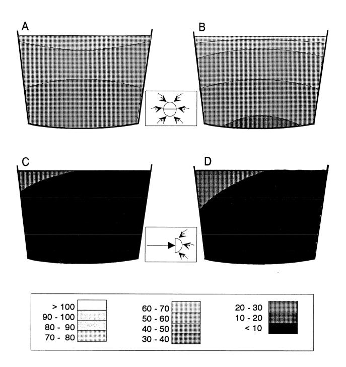
Fig. 3. Isolines of light intensities (relative values) measured in tanks with black walls and black bottom. A: clear water, 360°; B: green water, 360°; C: clear water, 180° (horisontal); D: green water, 180° (horisontal)
