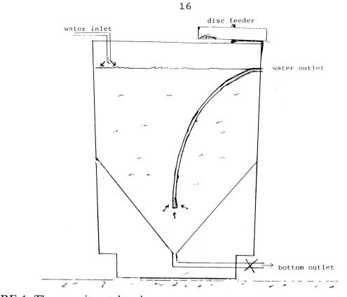
FIGURE 1: The experimental tanks
