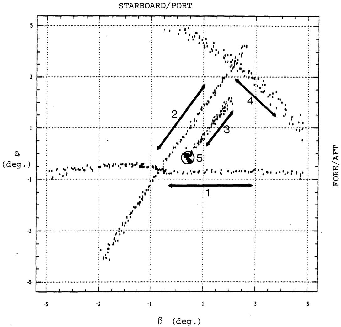
Figure 3. A plot of  $\alpha$  versus  $\beta$  gives the target position as seen by the split-beam echo sounder. The numbers one through five identify different paths of the calibration sphere. Note that track no. 5 was recorded with a nearly stationary target.
