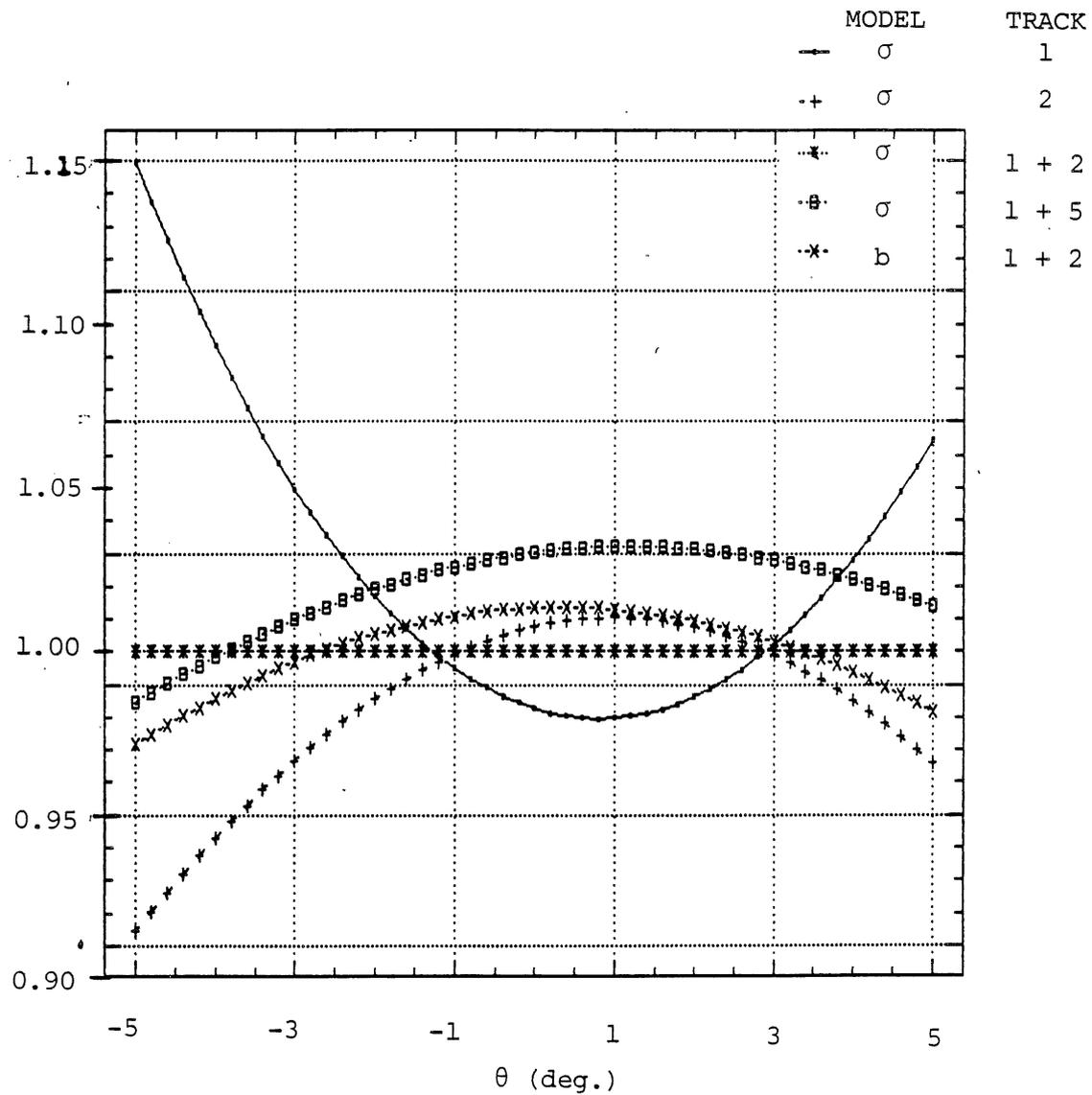
Figure 7. Relative calibration factors from equation 4, normalized with respect to data from track 1 + 2, using the backscatter model.
