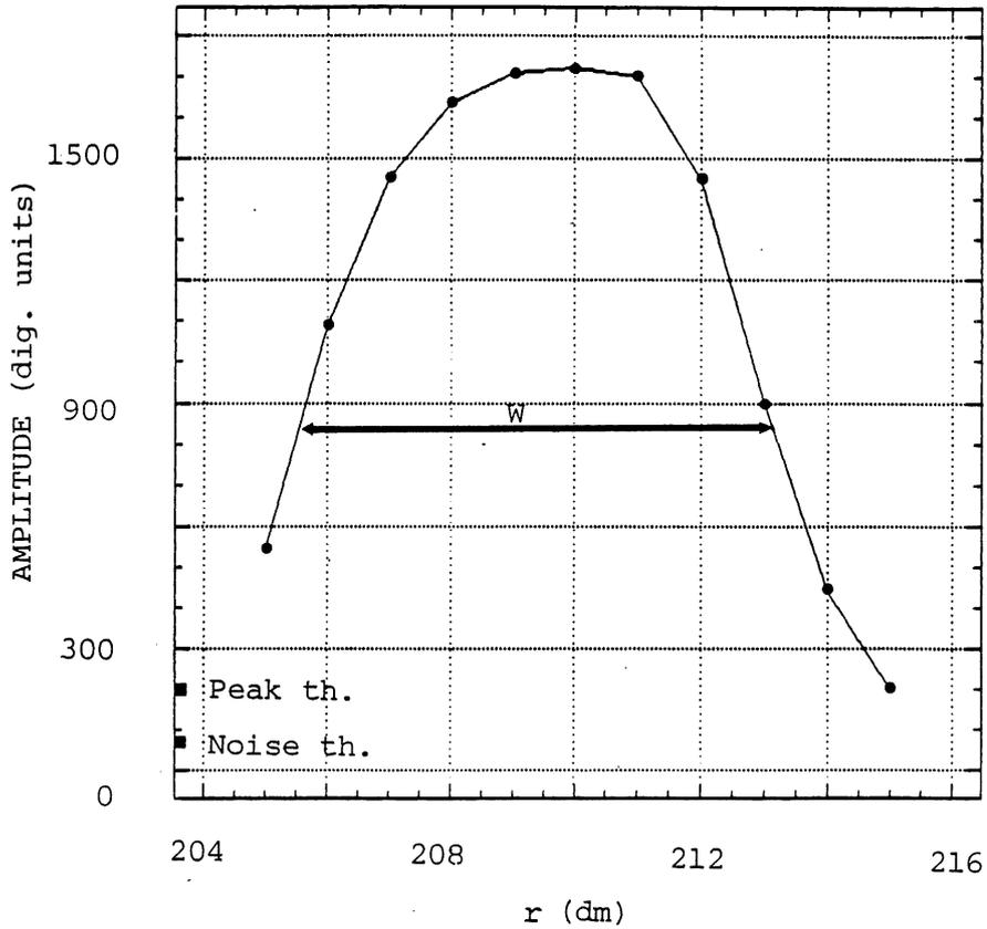
Figure 2. Single pulse from the sphere at 20.4 m depth. Only data above the noise threshold are collected. Small dots indicate actual data points, with angle data available on the rising part of the pulse. A single-target peak must exceed the peak threshold, and is characterized by the peak amplitude, width at half amplitude,  $W$ , angles  $\alpha$  and  $\beta$  and their standard deviation.
