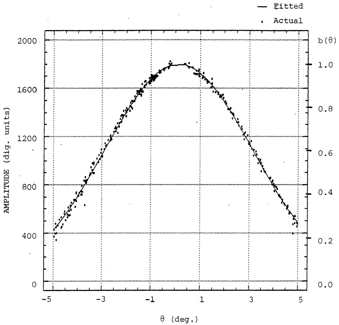
Figure 4. The approximate beam pattern, fitted to the data from track one and two.
