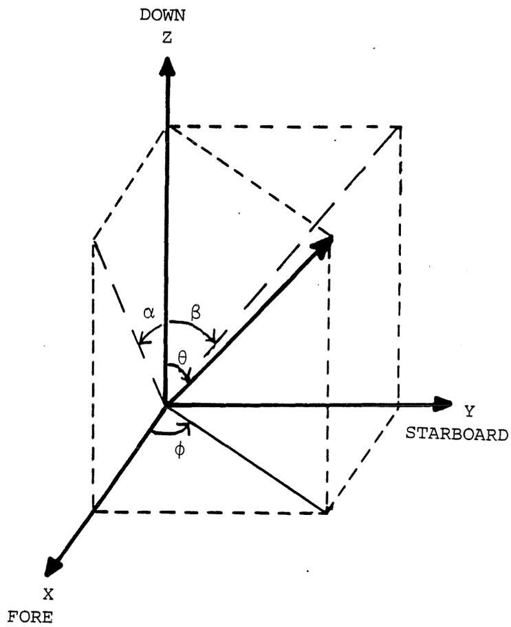
Figure 1. Used coordinate system. The fore/aft angle  $\alpha$  and starboard/port angle  $\beta$  are measured in the x/z and Y/Z plane respectively. Spherical coordinates  $\theta$  and  $\phi$  are also shown.
