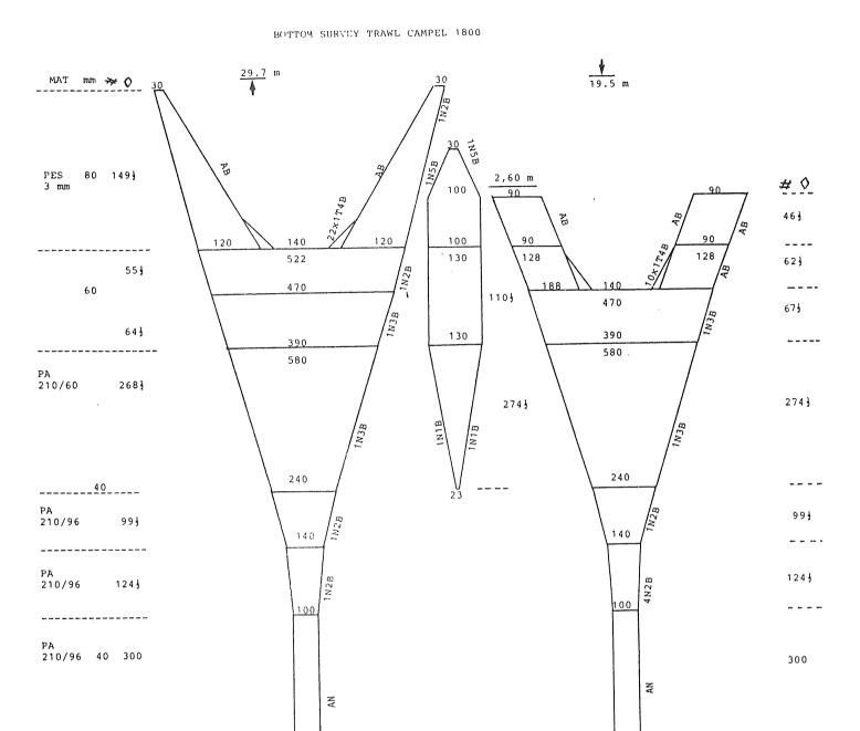
Fig. 1. Bottom survey trawl Campelen 1800.
