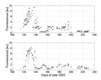
**Fig 8.** Comparison between observed FerryBox Chl Fluorescence (lower panel) and estimated chlorophyll for tracers starting from the Gabbard and drifting to the FerryBox route (upper panel)
