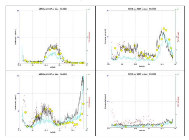
**Figure 10:** Comparison of the night (black) and day (blue) fluorescence, Chl-a (yellow) and the non-standard product FLH data (red) for some dates in 2004.(Upper left 24 February, upper right 9 March, lower left 16 March, lower right 29 June).
