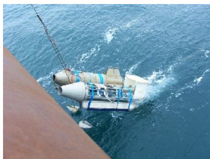
Figure 3.3.2.1: The frame, with both torpedoes mounted on top, as used for the comparing fishing trial.
