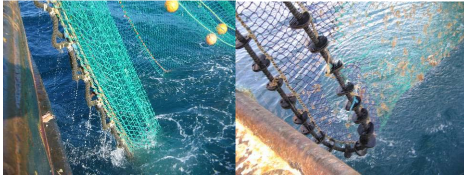
Figure 3. Examples of Grassrope and Rockhopper Footropes from seine nets
