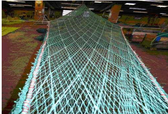
Figure 5. LMTP (800 mm) installed in the entire last tapered section.
