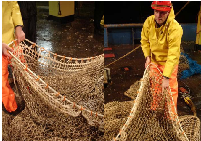
Figure 4. Benthos Release Hole inserted in bottom sheet of the port beam trawl, left the guider, right the escape hole
