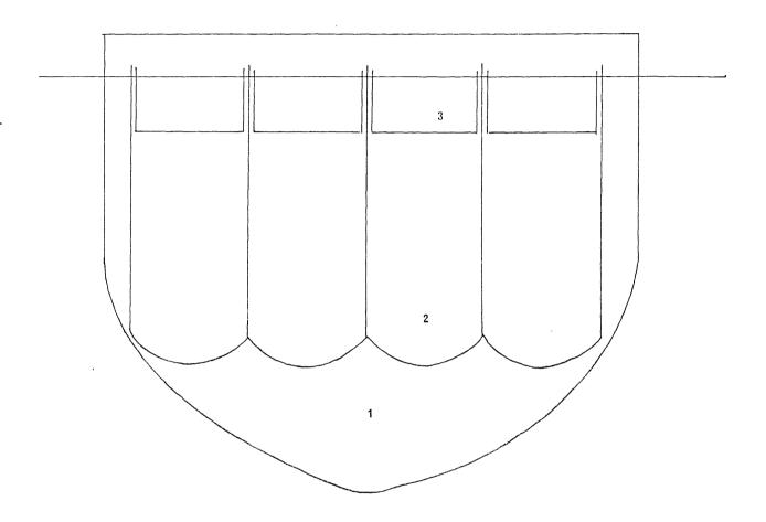
Figure 1. Pen arrangement. 1)Large production pen. 2)Incubation/start feed pen. 3)Plankton gauze bag.
