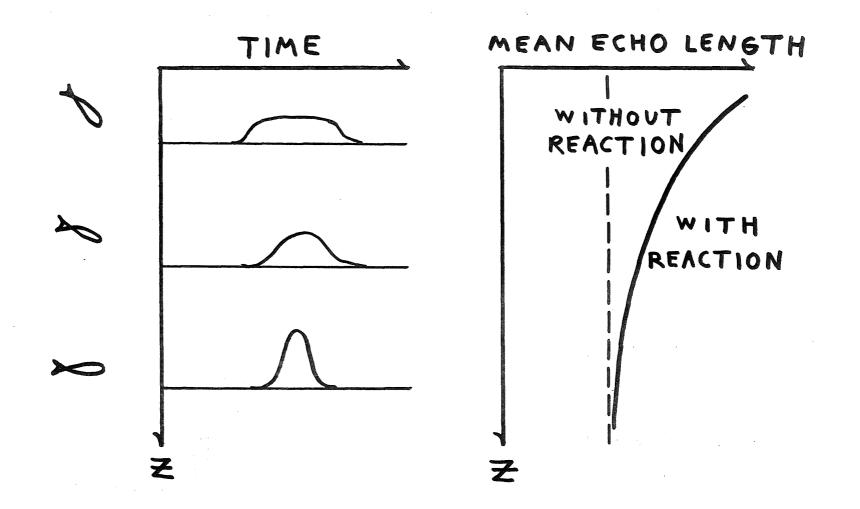
Fig. 2. Example of qualitative variation with depth z of mean echo length.
