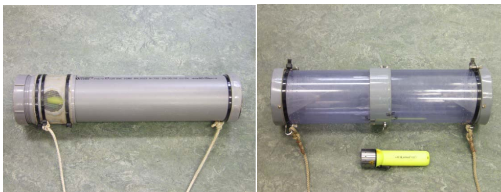
Figure NL.24 The two types of light traps used during the pilot studies in 2009 (left) and 2010 (left and right) to collect glass eel.
