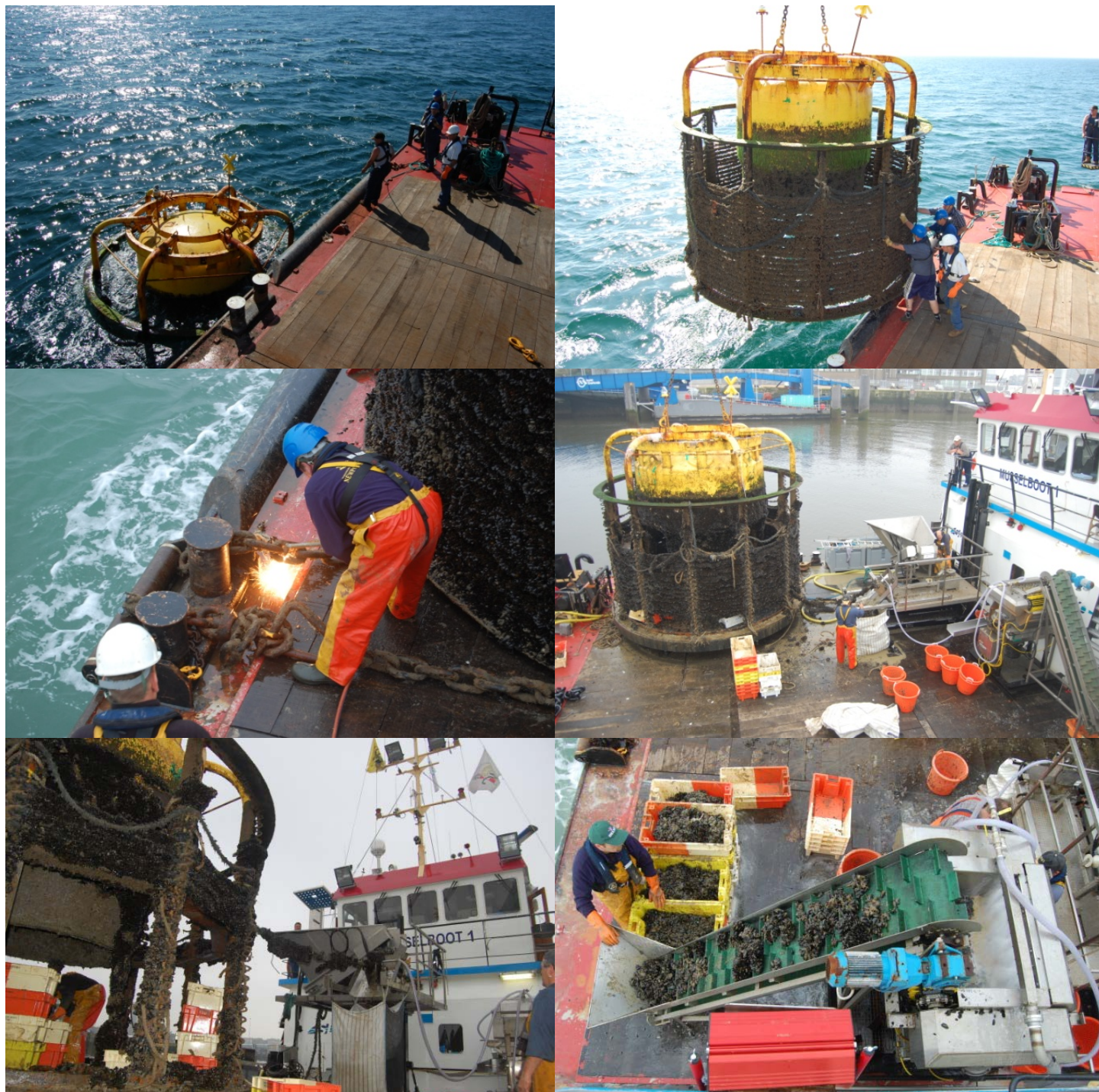
Figure 4.9. A series of pictures of the harvest of the SDVO buoys (photographs: ILVO, Kris Van Nieuwenhove).
