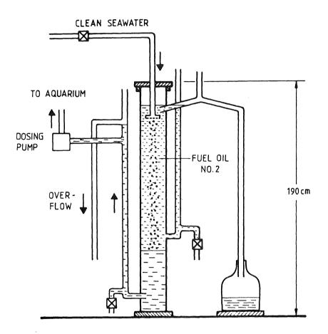
Fig. 2. The "oil column" for preparing seawater containing hydrocarbons
