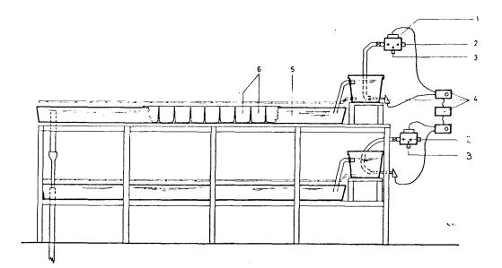
Fig. 2. The experimental set up. 1. The magnetic valve 2. Cold water 3. Warm water 4. The automatic system for controlling the valve 5. Water bath 6. Aquarium boxes.
