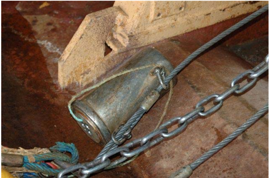
Figure 2.2.1.1: Wing canister for Scanmar mini-transponder shackled into the top bridle of the Campelen survey trawl at Northwest Atlantic Fisheries Centre in Newfoundland.
