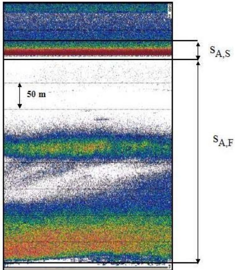
Figure 3. ER60 echogram taken in December 2002, showing the range and boundaries of  $s_{A,S}$  (397-427m for the transducer) and  $s_{A,F}$  (5-397m from the transducer).
