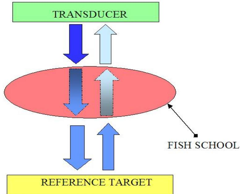
Figure 1. Scheme of the reference target technique for measuring acoustic extinction. The reduction in sound intensity is shown by the lighter colors in the arrows.
