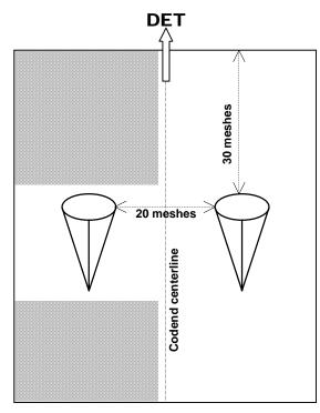
Figure 30: Layout of double Fish Eye installation.
