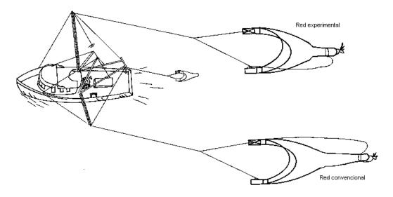
Figure 32: Paired Trawling Layout.
