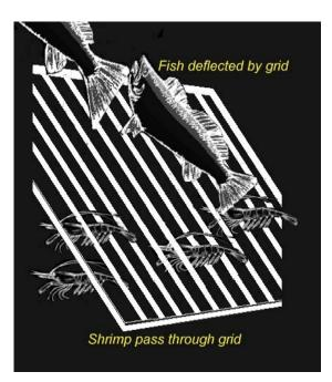
Figure 12: Schematic of Nordmore grid.
