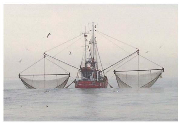
Figure 8: Typical twin-rig shrimp beam trawler.
