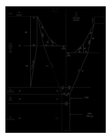
Figure 37: New shrimp trawl 13.50/15.70: RS-INP 1 (57 mm version).
