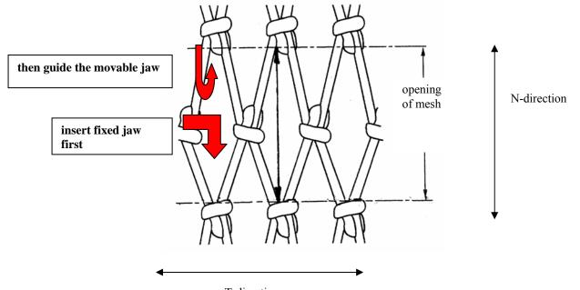
Figure 1: Insertion of the gauge. T-direction
