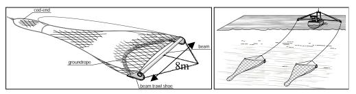
Figure 9: Schematic diagram of beam trawl.
