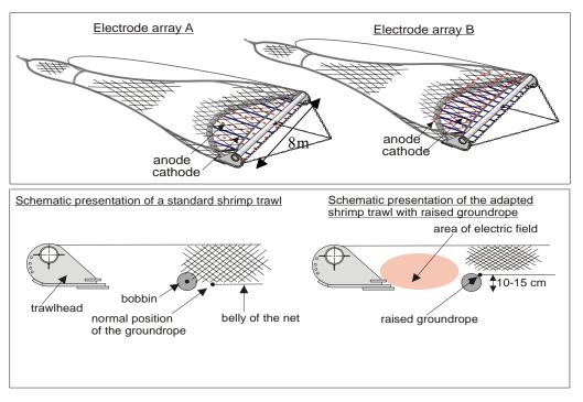
Figure13: Electric pulse beam trawl.
