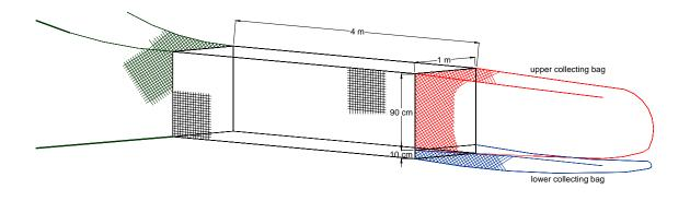
Figure 3: An illustration of the 1X1 m frame inserted in a square mesh aft shrimp trawl belly.
