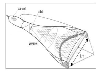
Figure 11: Schematic of sieve net.
