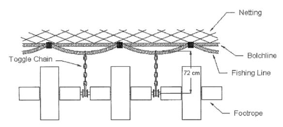
Figure 3: Schematic diagram of toggle chain attachment as per NAFO regulations.
