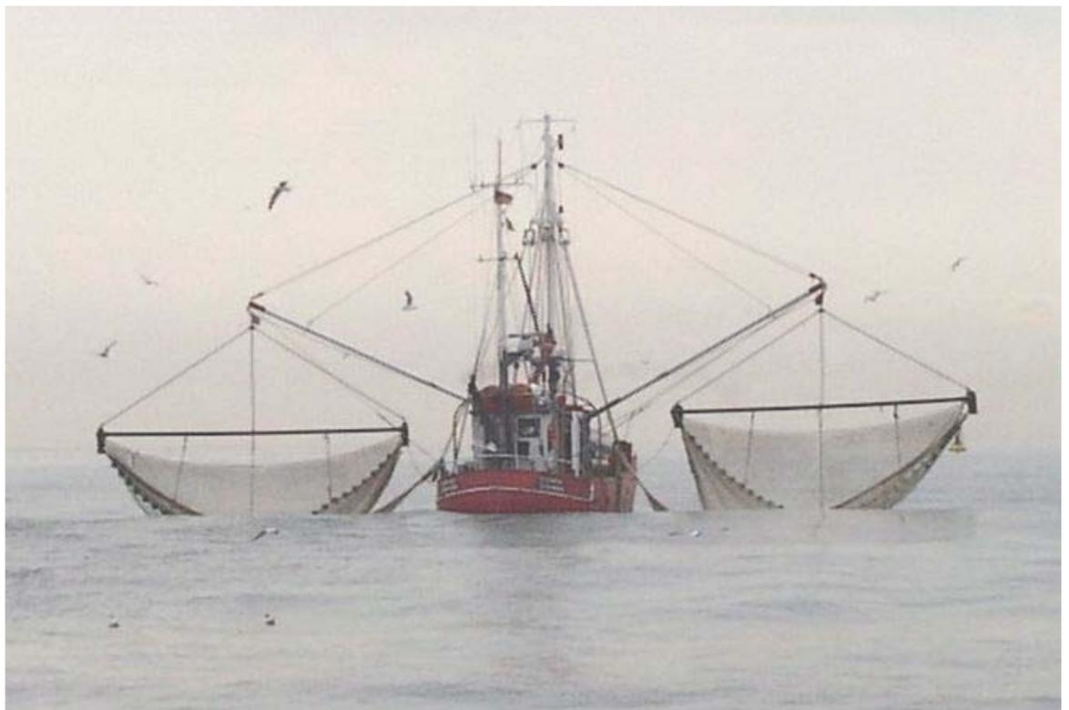
Figure 8: Typical twin-rig shrimp beam trawler.
