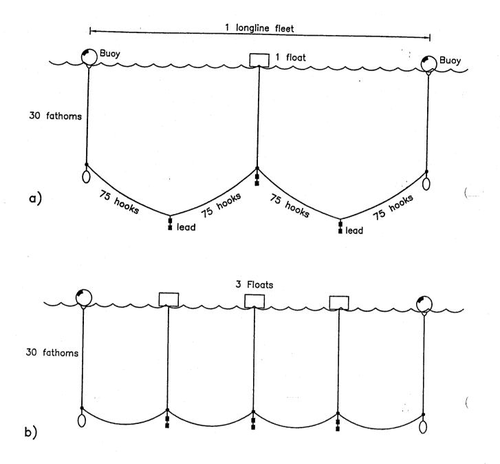
Figure 2. Rigging of the longline fleets. Vessel II used both method a) and b) in 1995, while vessel I rigged as b) with 100 hooks between the floats. In 1996 both vessels used the last method.
