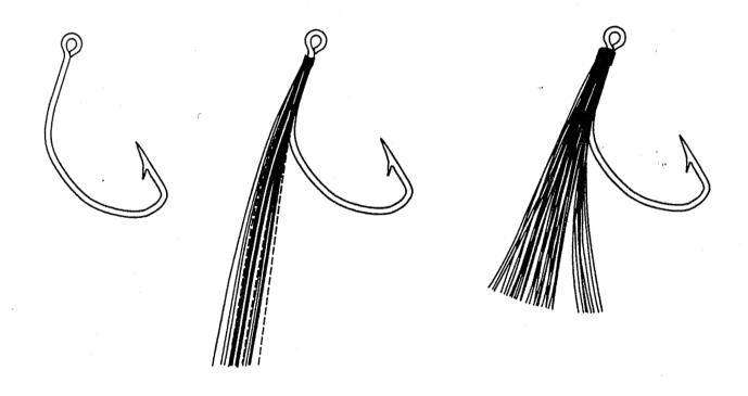
Figure 4. Eagle Claw 1607 hooks without (a), with white (b) and red (c) nylon bristles attached to the hook shank.
