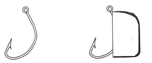
Figure 3. Mustad Wide Gap 5 hooks with and without an inedible plastic body attached to the hook shank.
