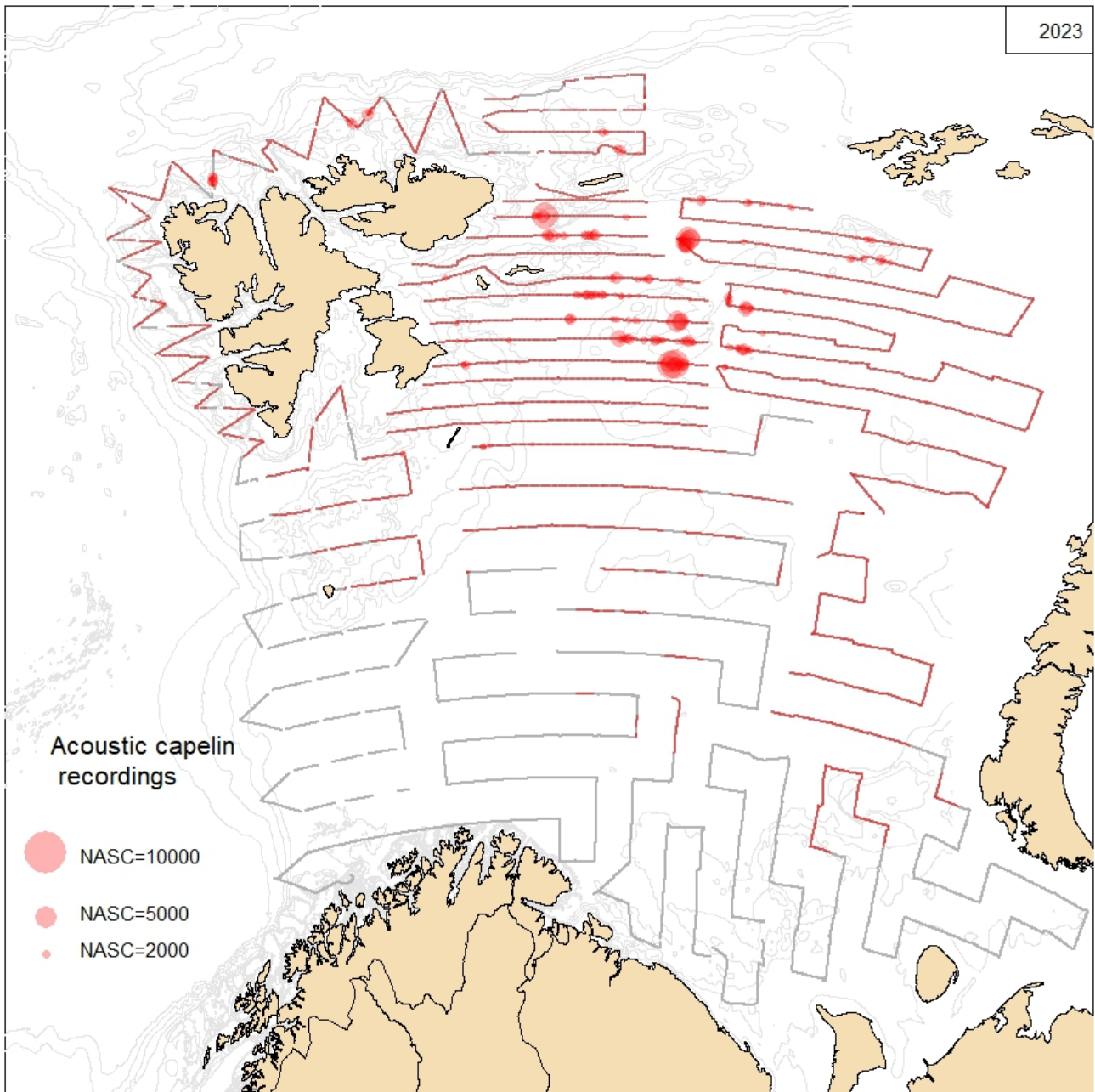
Figure 10.1. Survey coverage and geographical distribution of acoustic recordings of capelin in autumn 2023. The size of the circles corresponds to nautical acoustic scattering coefficient (NASC; m^2/nmi^2 ) per 1 nautical mile. Gray dots mark transects or transect sections without capelin recordings.
