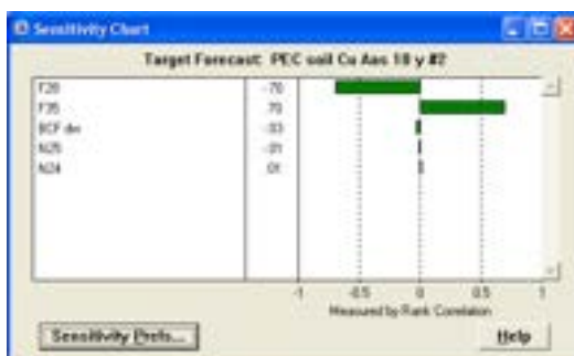
Figure AVIII-23 a,b,c,d. Forecast of PEC soil for Cu. a) Frequency distribution b) statistics c) percentiles d) sensitivity chart, where N25 is TF wheat, N24 is TF oats, BCF DW is TF barley, F28 is precipitation, F35 is Kd. Default PEC soil value Cu is 15.89 mg kg -1 DW.
